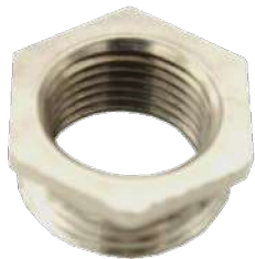
#74 Reducer 1/2"IP Outside Thread x 3/8"IP Tap x 7/16"H Nickel Plated Reducer 7/8" Across Flats
