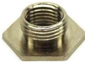
Hex Flange 3/8 - 1/4 3/8"IP Outside Thread x 1/4"IP Tap x .367" H Nickel Plated Reducer 1" Across Flats
