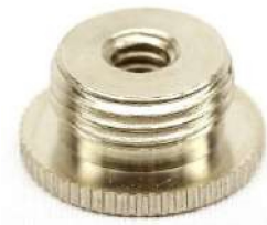
A3/8IP x 1/4-20 F Adapter 3/8 IP male x 1/4"-20 female .885" W x .426"H x .325" 3/8"IP thread
