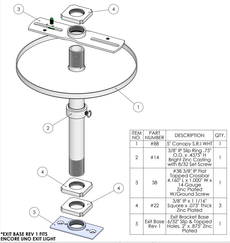
STEM LENGTH WILL VARY. ORDER SEPARATELY C515-E REV 1 USED WITH STEM 3/8" IP 3/8" IPS .625"-.635" O.D. 18 T.P.I.
