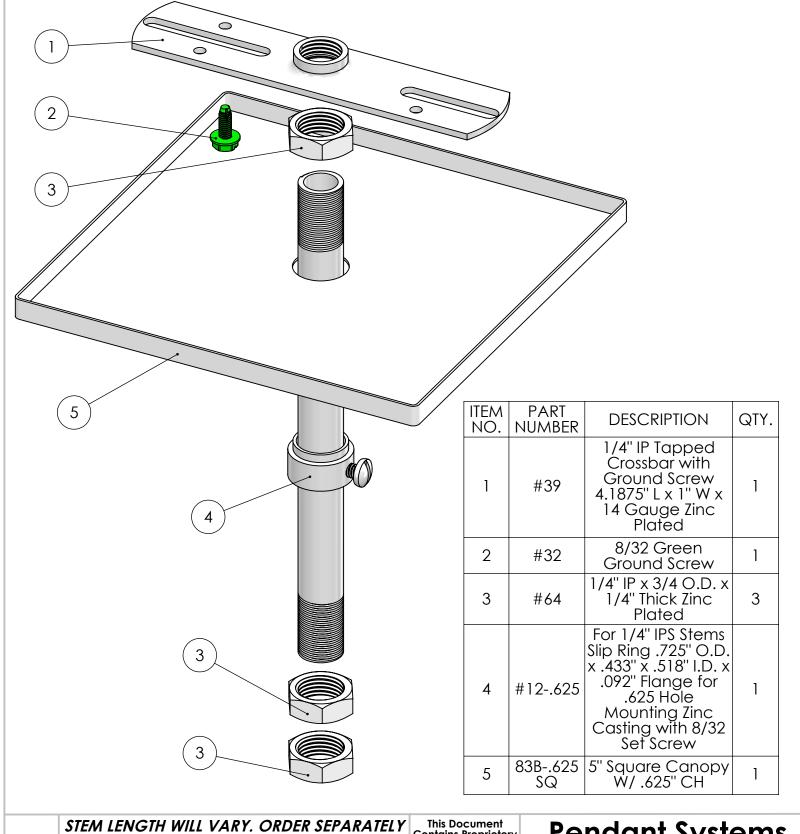
C416 SQ USED WITH STEM 1/4" IP 1/4" IPS .500"-.510" O.D. 18 T.P.I.
