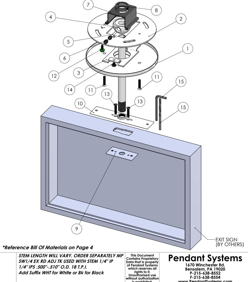
is prohibited. www.PendantSystems.com \*50° SWIVEL UNLESS OTHERWISE SPECIFIED DIMENSIONS ARE IN BOTH INCHES & MILLIMETERS UNLESS OTHERWISE NOTED TOLERANCES: TITLE: MP-SW1/4 EX RD ADJ TK LINEAR: XX= .02" XXX= -.010" ANGULAR: + 1 Degree DO NOT SCALE DRAWING MATERIAL: Part # DEBUR AND BREAK SHARP EDGES REVISION SCALE: NTS SHEET 1 OF 4 DRAWN DATE: 9/27/16 Drawn By: MWR
