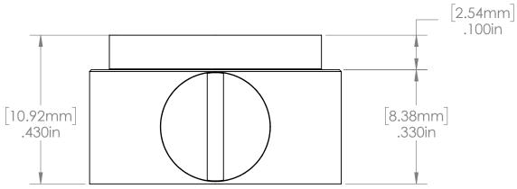
For 1/4" IPS Stems Slip Ring .725" O.D. x .430" H x .550" I.D. x .092" Flange for .625" Hole Mounting Zinc Casting w/ 8/32" Set Screw
