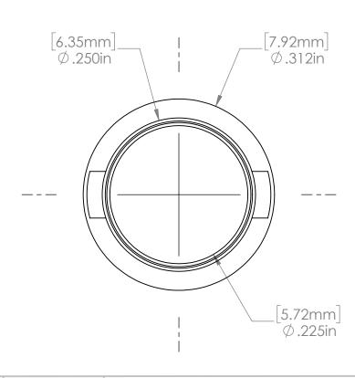
1/4" Hole Plug .3125" H Used to plug large side of keyhole for Cross Cables with Half Ball End fittings
