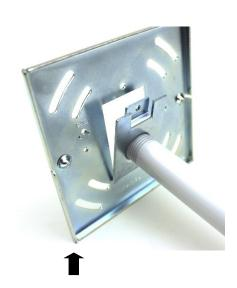
Insert Tail End then shift tapped side on inside of crossbar and fasten with 8/32" screw
