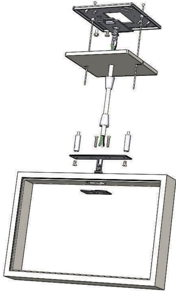
**Assembly is rated for 50 Lbs. Static Loads Only (No dynamic or moving loads)**
