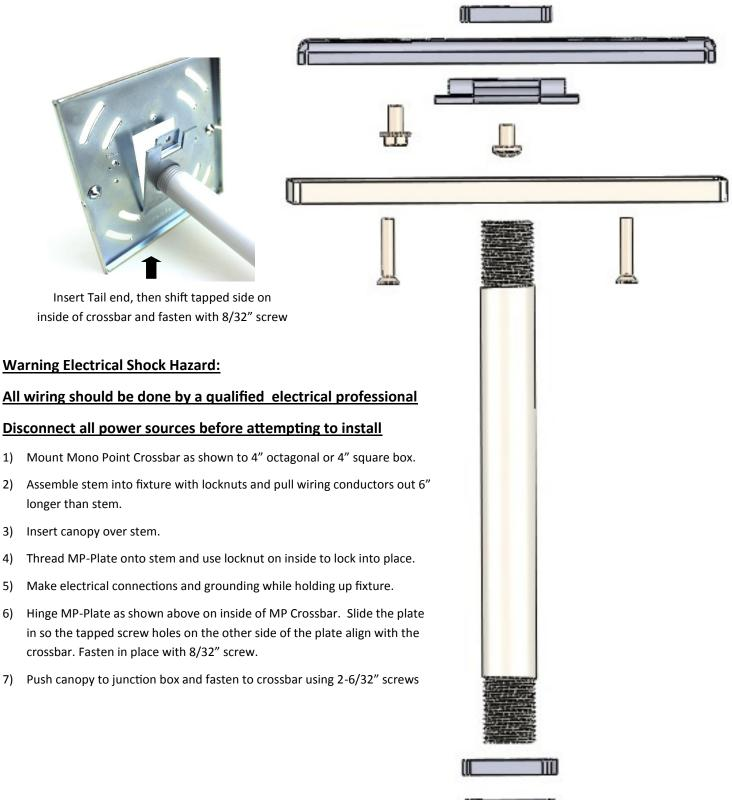
Assembly is rated for 50 lbs. Static Loads Only (No dynamic or moving loads)
