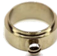
#142- 1/2"IP Slip Ring Nickel Plated W/8/32" Screw Add suffix PR Wht for White or PR Blk for Black 1.04"W x .426"H (including Flange) x .850"ID .925"Flange
