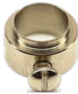
#12-.625" -1/4"IP Slip Ring #12-.625 for 1/4" IPS Stems Slip Ring .725" OD x .433" x .518" ID x .092" Flange for .625"Hole Mounting Zinc Casting w/8/32" Set screw
